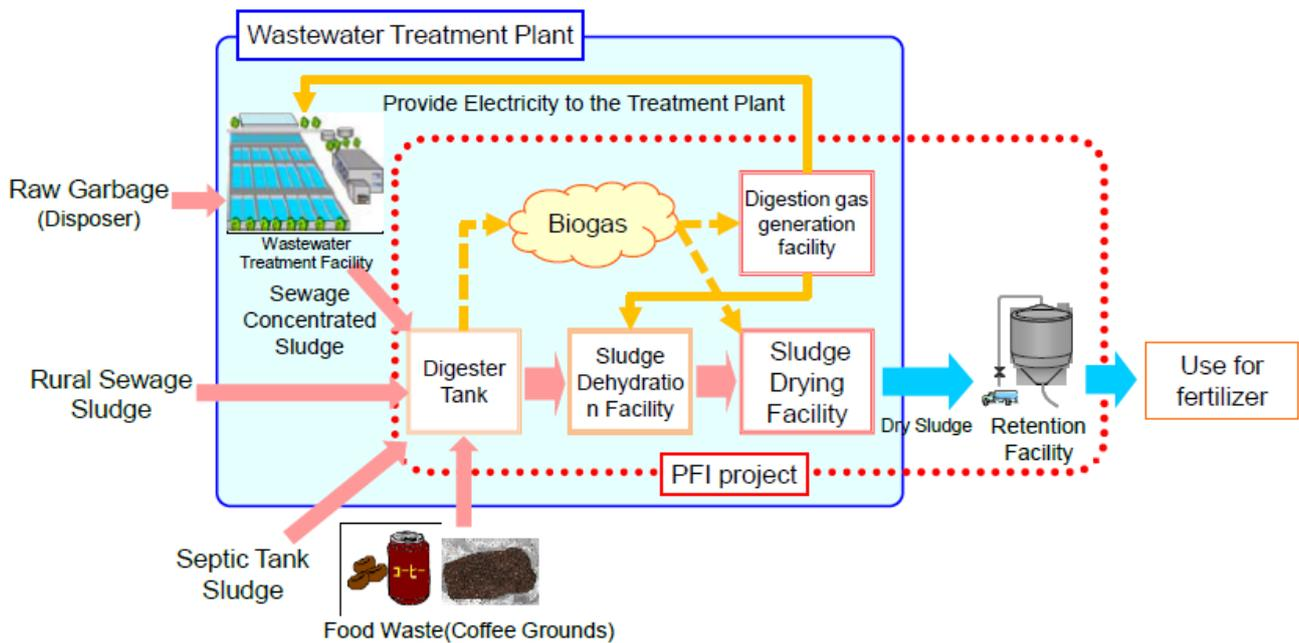
Figure 10 Schematic of Project
