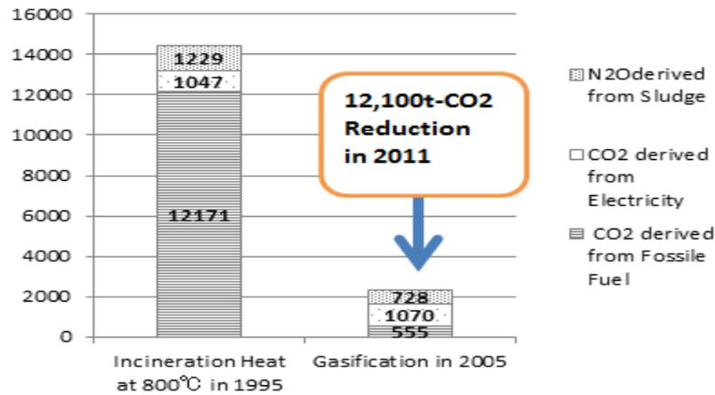
**Figure 6 Comparison of GHGs emissions between incineration and gasification**
