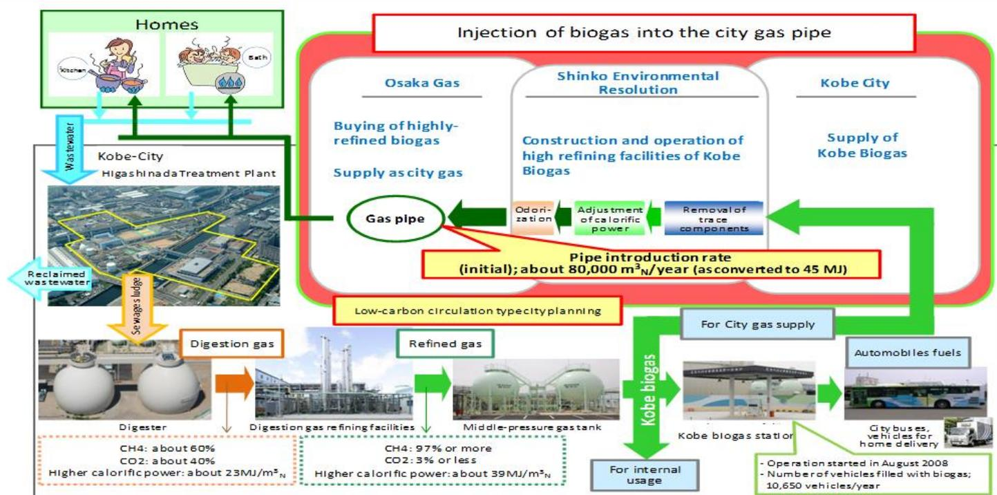
Figure 7 Biogas Purification at Kobe WWTP
