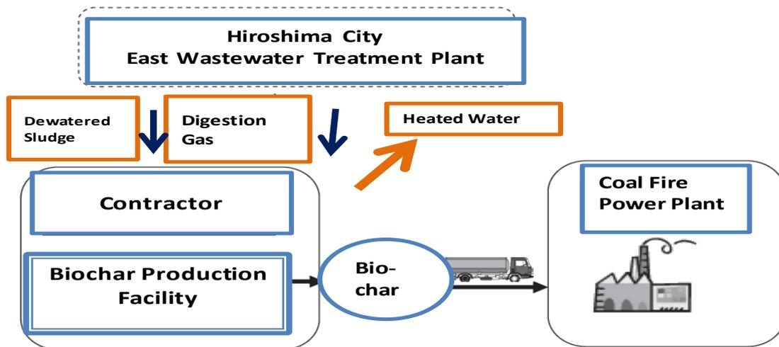
Figure 3 Schematic of Project
