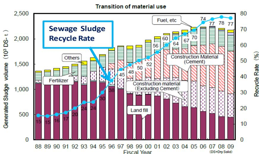
Figure 1 Trend of Sewage Sludge Recycle
