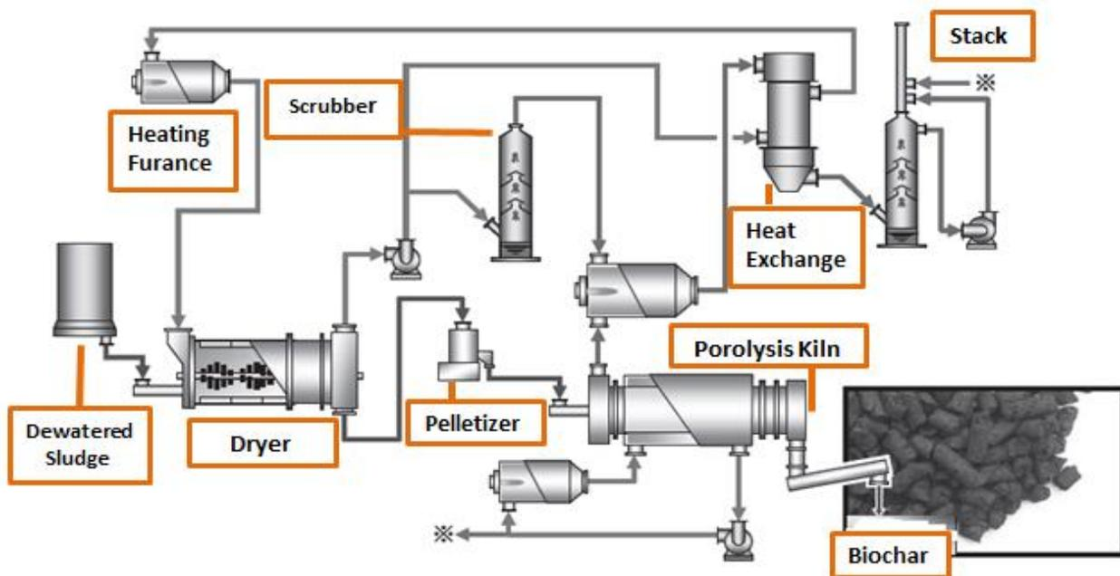
Figure 4 Flowchart of Low Temp Biochar Production System
